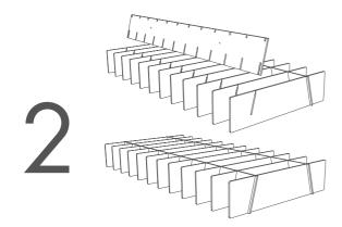
Once all the fins are inserted into the rail, flip the Lattice over 180°. Slide the remaining rail into the slots on the fins; again ensuring the tabs on the fins click into the groove on the rail.
