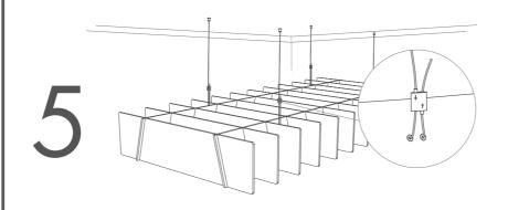
Lift the Lattice up to meet the cables and loop the wires through the plugs followed by the "Velda" cable clips.
