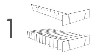
Lay one rail on its edge with the long slots facing up and methodically slot the fins into each slot on the rail at 90 degrees. Make sure the tabs on the fins click into the groove on the bottom of the rail.
