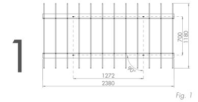
Determine where you want the Lattice to hang (Fig. 1). Mark the ceiling mount points as per the above diagram.
