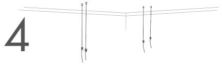
Screw assembled cables into the fixed ceiling mounts. Decide which way up the Lattice will hang - convex down or convex up - and lay the rails out in their
