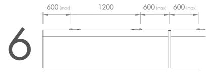
Final position of Frontier Connectors should be no more than 600mm from edge of fins.
