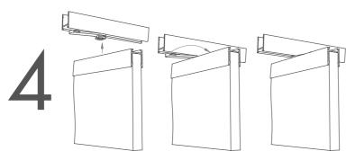
With Frontier Connector perpendicular to the Channel, snap Channel onto Connector. Once position is confirmed, rotate Connector 90 degrees to lock.
