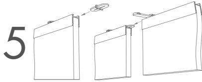
If two fins join, insert a Frontier Joiner into the first (locked) Channel. With the attaching fin's Connectors snapped but unlocked, slide the Channel onto the Joiner before locking Connectors.
