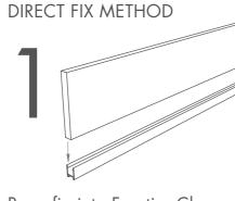
Press fin into Frontier Channel, using a rubber-faced hammer to ensure a snug fit.
