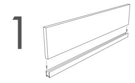
Press fin into Frontier Channel, using a rubber-faced hammer to ensure a snug fit.
