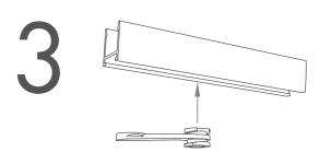
With Connector co-linear with support rail, snap Connector into extrusion in approximate position.
